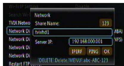
TViX allows selecting 10/100 and Gigabit network. For the Gigabit network to function, a CAT6 network cables is mandatory. Both SMB and NFS are featured and can
