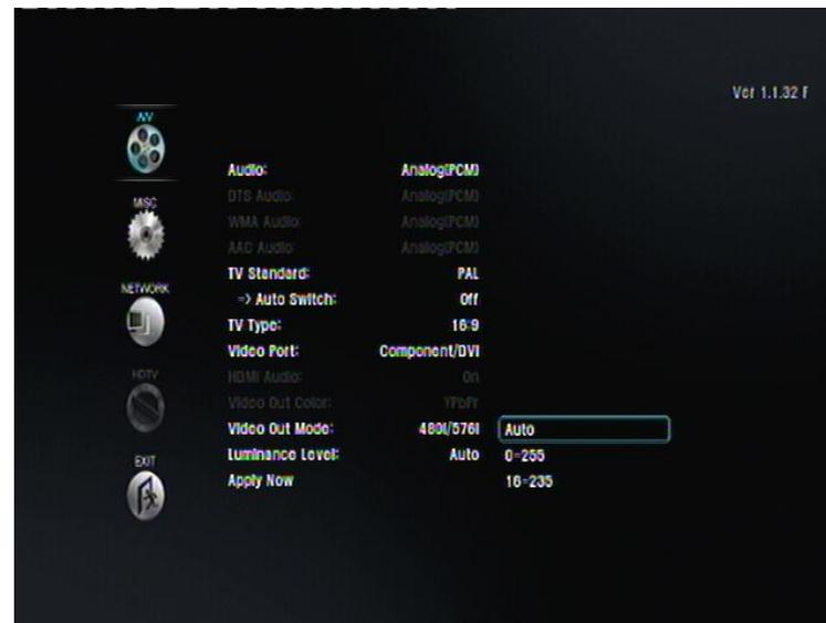
New is the "Luminance" mode where you can select between the usual 0-255 (PC Black White levels), 16 – 234 (Video Black White levels) and an Auto Mode where the TViX will be following up on information that the display provides to TViX through HDMI
