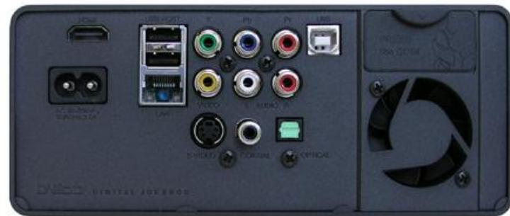
The little cover on the upper right, can be removed making room for a DVB-T tuner (the T430) allowing the unit to become a recorder for free to air sources.
