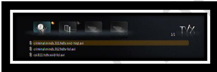
The upper 4 icons respectively provide connectivity to Internal HDD, Network sources, USB1 and USB2 which are grayed out since no USB sources are connected. Important to know for all HDD users is NTFS is supported whilst using external hard drives. This is not always the case with media players, but is becoming the norm for newer models launched.
